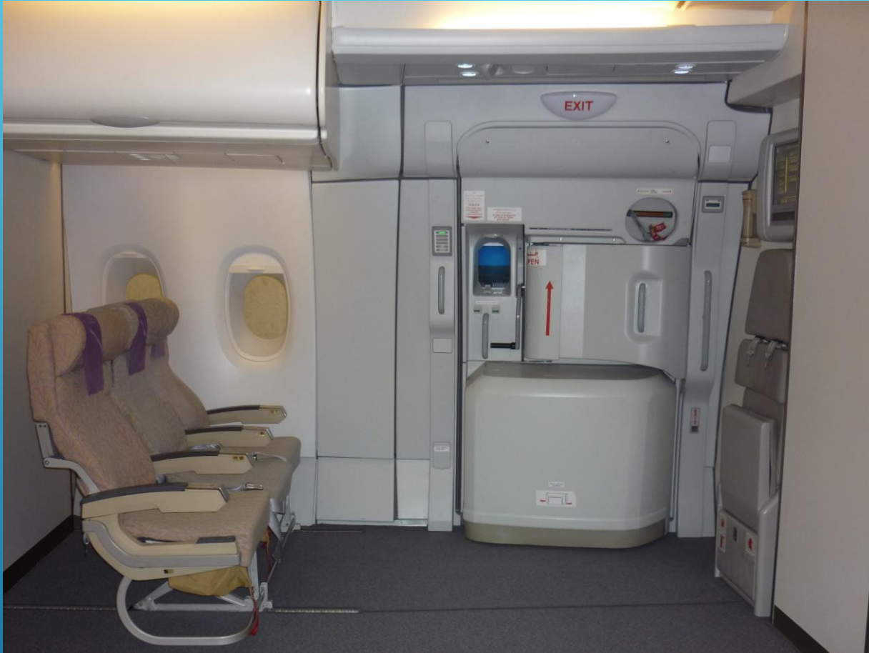
Main Deck Door LHS – Door bustle containing slide/raft
